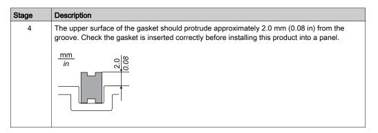
The gasket must be inserted correctly into the groove for moisture resistance for this product.
